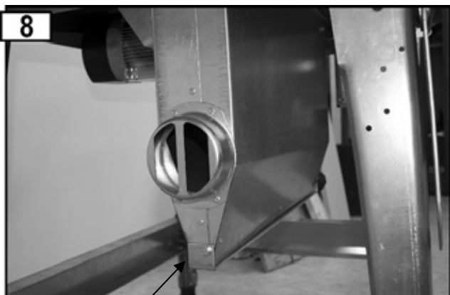
Chip ejector slot closed (operation with chip extractor)
