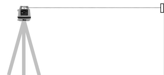
To reach a slope of 3% the receiver must be displaced down for 30cm and attached.
